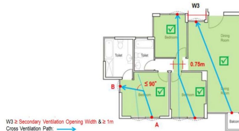
Figure 14 Openable Windows Locations and Cross Ventilation Path (Rooms with cross ventilation potential are indicated with a tick)
